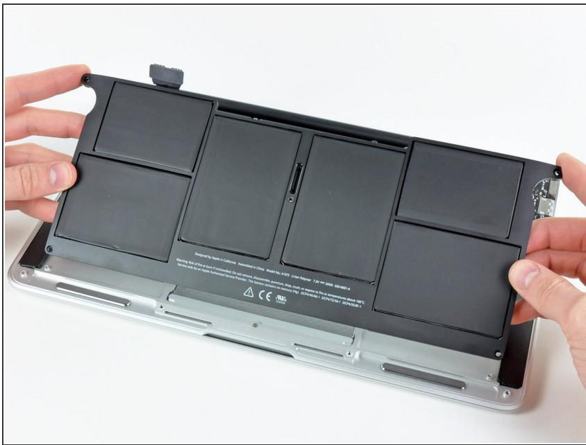
**⚠** When handling the battery, avoid squeezing or touching the six exposed lithium polymer cells.
